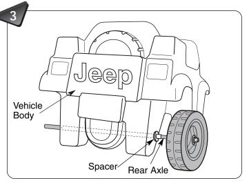
• Insert the rear axle through the holes in the rear of the vehicle body. Make sure the spacer fits into the hole in the vehicle body.
